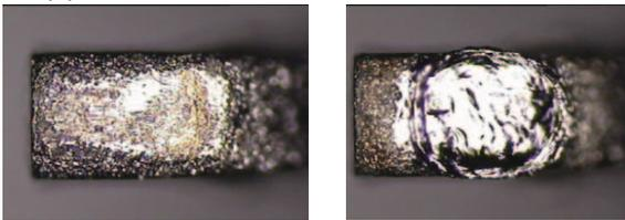
**Figure 6.** SEM image of the ablated sample area on the lead.
